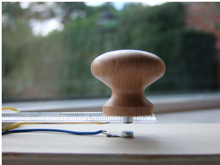
Figur 12. To loddefliger monteres under skruerne.
