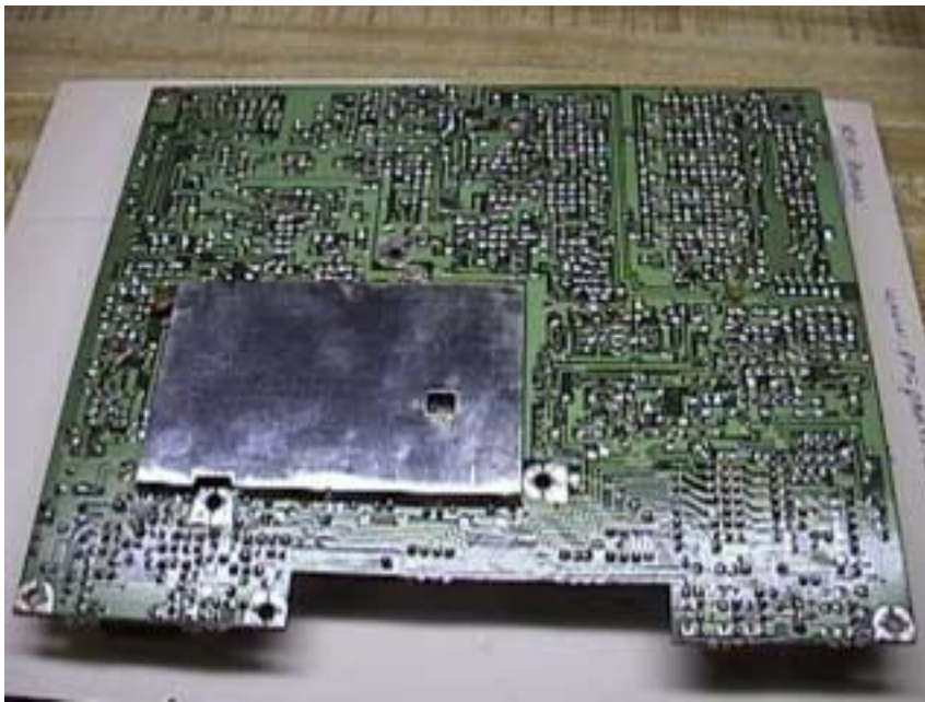
RF board removed (solder side) with shield.
